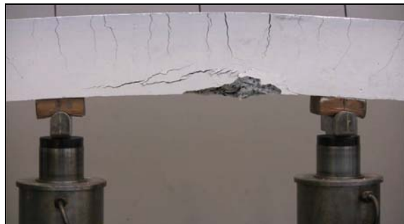
Figure 2. Extract from video available at YouTube [6], showing beam behaviour at failure.
