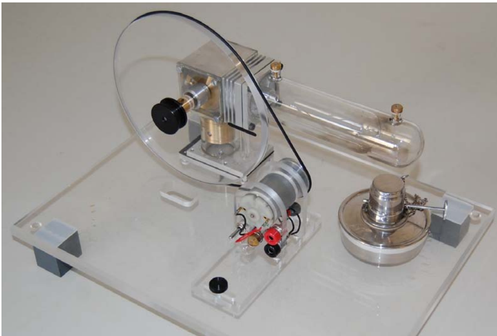
Figure 3. Transparent Stirling engine used for second assignment
