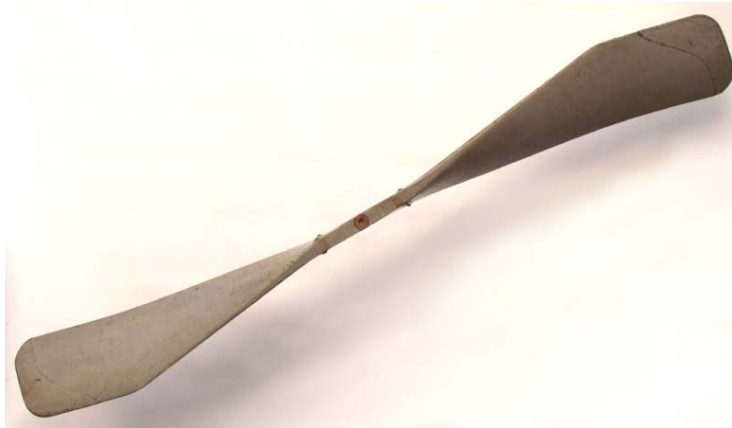
Figure 3: The Wright propeller, a near optimal design based on knowledge acquired through testing [10].
