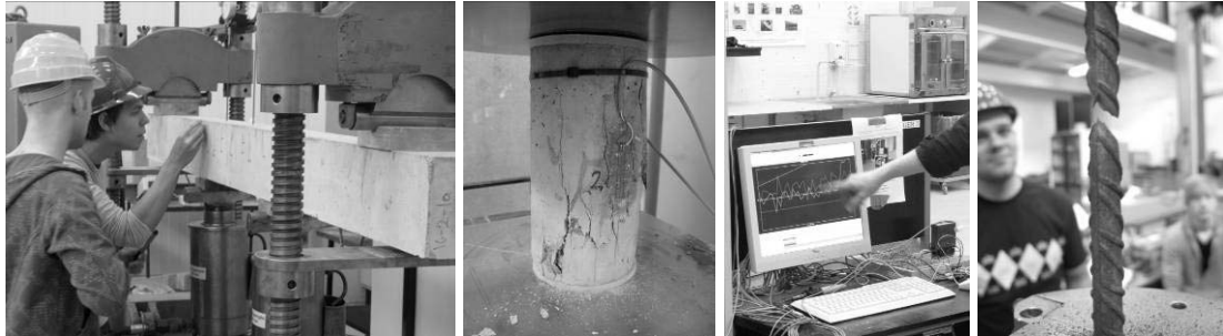
Figure 4. From left to right: beam testing, concrete compression strength test, data acquisition, steel tensile strength test. Photos: Holger Koss.
