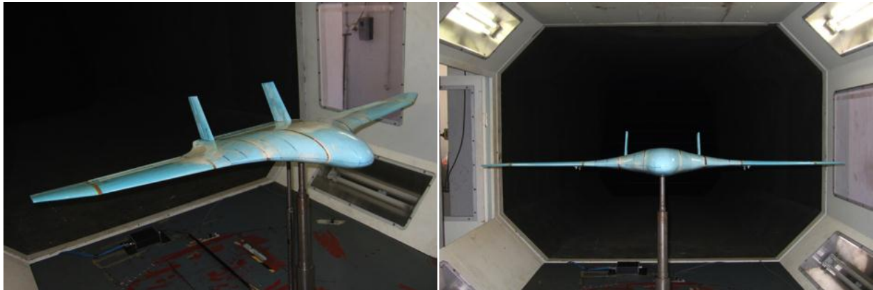
Figure 5. Half-scale wind tunnel model installed in the 7 by 5 ft wind tunnel in Sydney.
