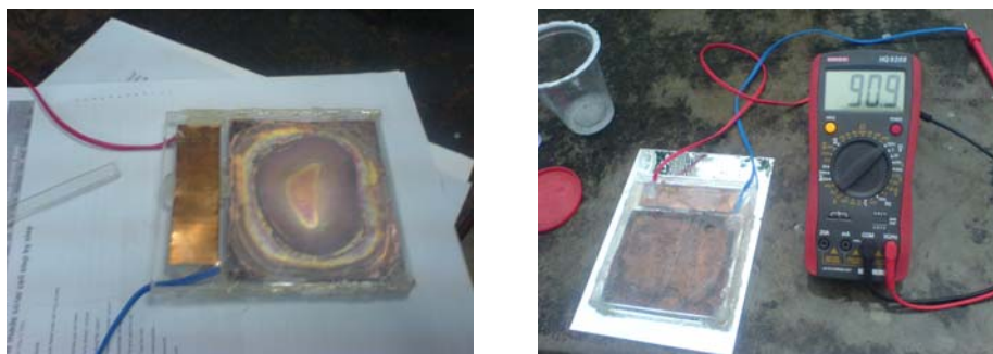
Figure 1. Solar Photovoltaic Cell (left) and Testing of the Cell (right)
